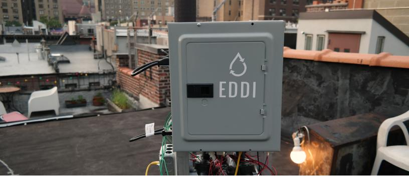
To address this issue, we built an ElectroDialysis Desalinator for Irrigation, affectionately known as EDDI. In Electrodialysis, an electric field is used to separate salt ions from the water, producing low-salt water that is ready for irrigation. While desalination is not a new concept, we are approaching it from a different angle by putting the technology for it directly into the hands of the farmers that are impacted the most by low-quality groundwater.
